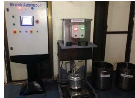
Fig.1. Experimental setup of automated precise liquid transferring system
