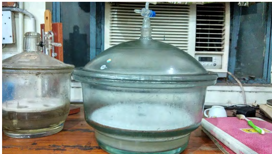
Fig. 27: Desiccator containing K 2 SO 4 at the bottom
