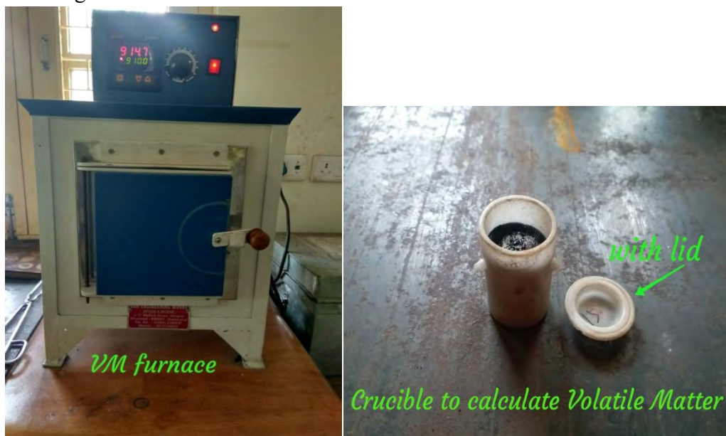
Fig. 19:Muffle Furnace (or Volatile Matter furnace) Fig. 20Crucible to calculate Volatile matter
